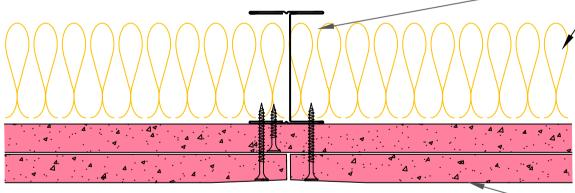
2x15mm British Gypsum Gyproc FireLine fixed with SPEEDLINE Drywall Screws at 300mm centres (200mm centres at external angles). Ref to table for fixing length.
